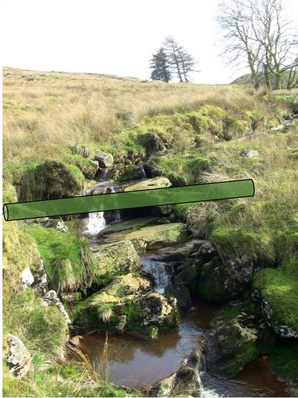
Figure 13. Nominal pipe location for an above-ground crossing. The metal sleeve pipes would be painted with a suitable drab colour such as Halfords ultra matt camouflage green https://www.halfords.com/motoring/paints-body-repair/specialist-decorative-paints/halfords-camouflage-spray-paint-green-300ml .
