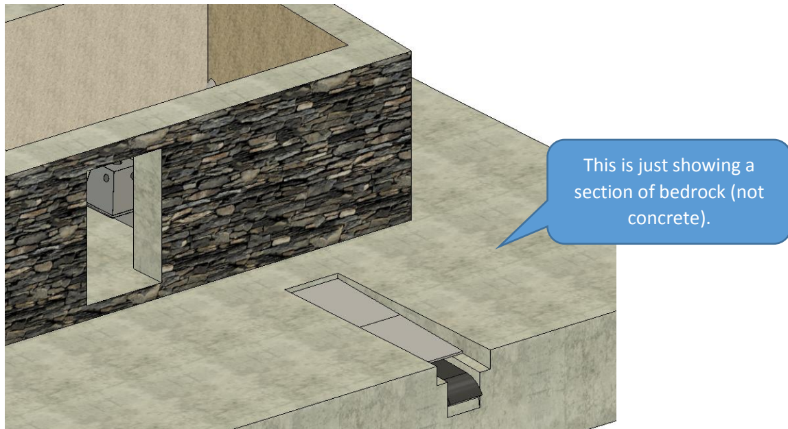
Figure 20. Tailrace will be cut into the stream bank (bedrock) as a channel with slate covering plates (900*600*20 mm), then recovered with soil and turf (not shown). Channel cross-section 360 mm * 150 mm. Water then flows down the bank like any other tributary joining Afon y Foel from the side.
