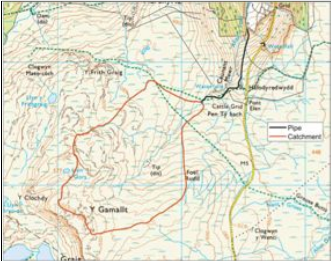
Map 1: The penstock is marked in black with the HEP catchment in brown.
