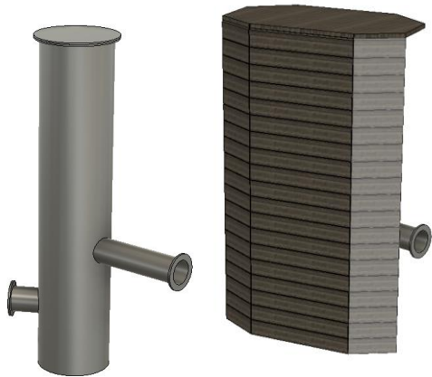
Figure 7. Settling tank (a) pipe section, (b) cladding to hide it.
