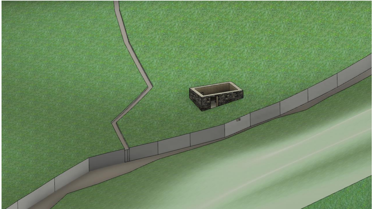
Figure 18. Hut will be partially built into the slope. Tailrace returns water to Afon y Foel.
