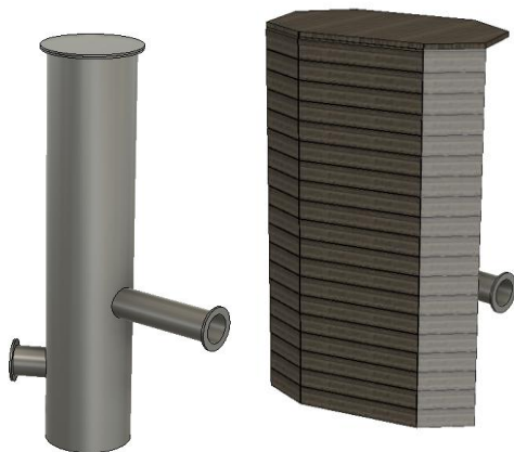
Figure 16 (a) Settling tank construction, (b) appearance of wooden fencing cover.
