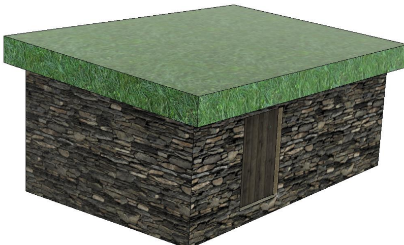
Figure 19. Turbine hut appearance. Wall dimensions (external) 4.6 m long \times 2.8 m wide \times 1.5 m high (floor to ceiling). Turf roof.
