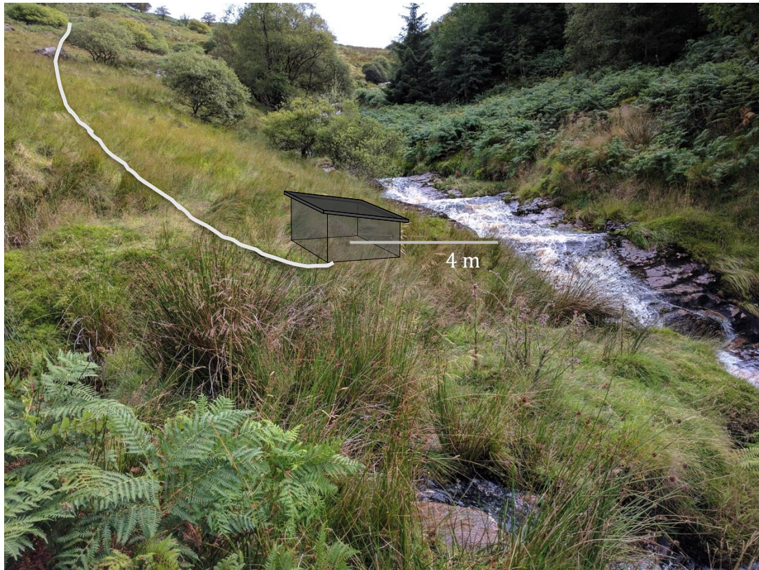
Figure 4. Proposed turbine hut (very roughly to scale), built into the slope & mostly hidden from the road. 3 m × 1.5 m × 1.5 m high internally, single-pitch slate roof, stone walls + internal insulation, 4 m × 2.5 m externally. Grey bar to show scale.
