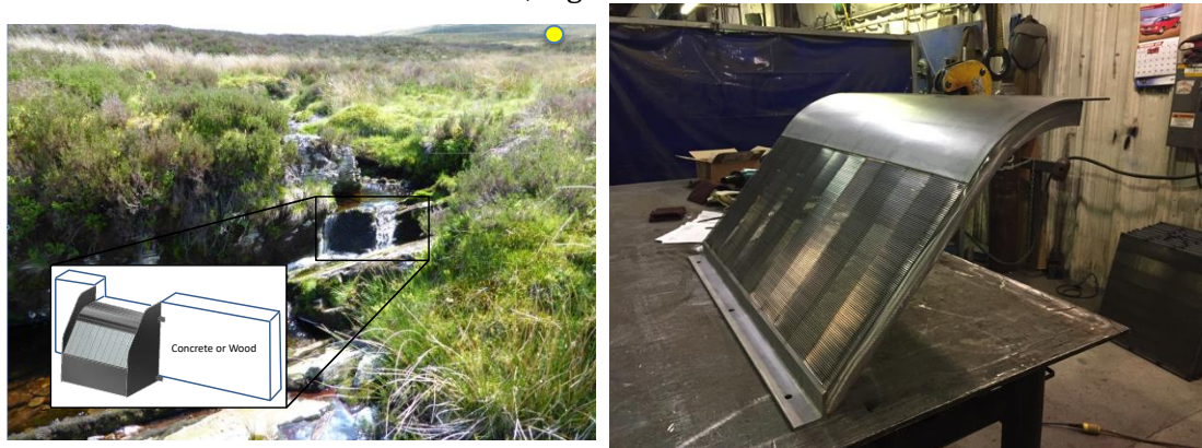
Figure 2. Possible Coanda screen installation (a) Elgin screens box CBS0.50-1 (their drawing). The side buttresses would probably be just a concrete lip to raise the bedrock by \approx 60 mm to ensure water did not bypass the box in dry weather. (b) Screen that (with rear collector) could be bolted to bedrock – probably at a smaller scale than this.
