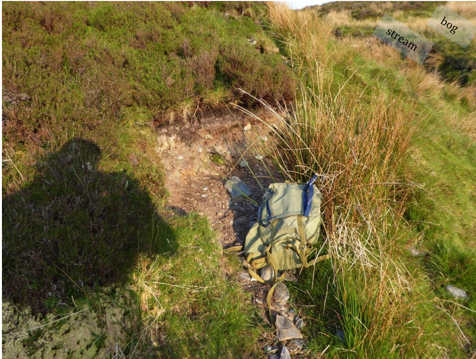
Figure 20 (Fig. 38 from the pre-application geomorphology survey, location “x” in Fig. 19). Soil characteristics. The pipe route will as far as possible pass through well-drained soil. (The blanket bog in the background, as marked in Figure 19, is drained at its lower edge by two small streams. The pipe route passes below the confluence of these and will thus have no impact on the blanket bog region).
