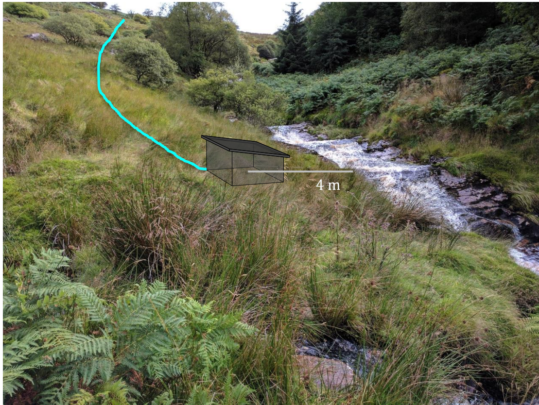
Figure 7. Proposed turbine hut (very roughly to scale), built into the slope & mostly hidden from the road. 3 m × 1.7 m × 1.5 m high internally, shallow-pitch turf roof, stone walls + internal insulation, 4 m × 2.7 m externally. Grey bar to show scale.
