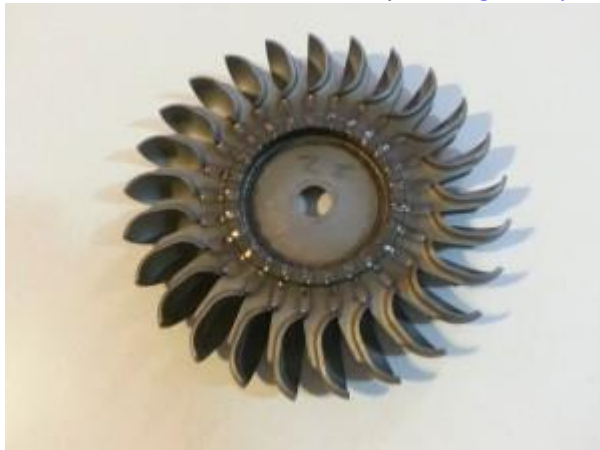
Figure 17. Stainless steel Turgo runner.
