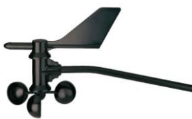
Figure 15. Appearance of a typical anemometer (18" long by 5" wide)
