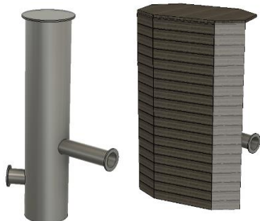
Figure 14. (a) Settling tank construction, (b) appearance of wooden fencing cover, (c) view looking upstream. The tank will be insulated to avoid freezing and hidden behind a shiplap fencing panel.
