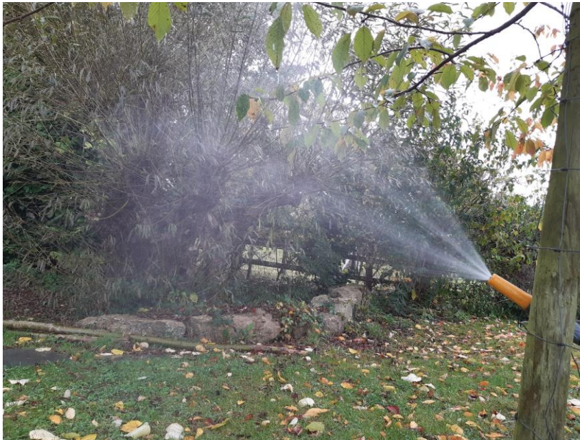
Figure 4. Demonstration of the mist obtained from a 0.05 L/s spray. This is with 3 bar pressure; at 1.5 bar (15m head) the spray would be slightly coarser and would take longer to evaporate.
