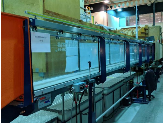
Figure 11. Tilting flume (300 mm wide, flows up to 32 litres/sec).
